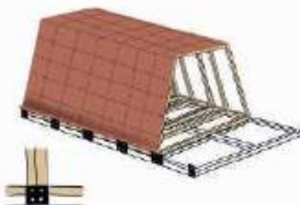
**EN** The base structure is made of treated wood beams for outdoor use, with transverse reinforcements made using a nesting system developed in Japan thousands of years ago and still in use today.
